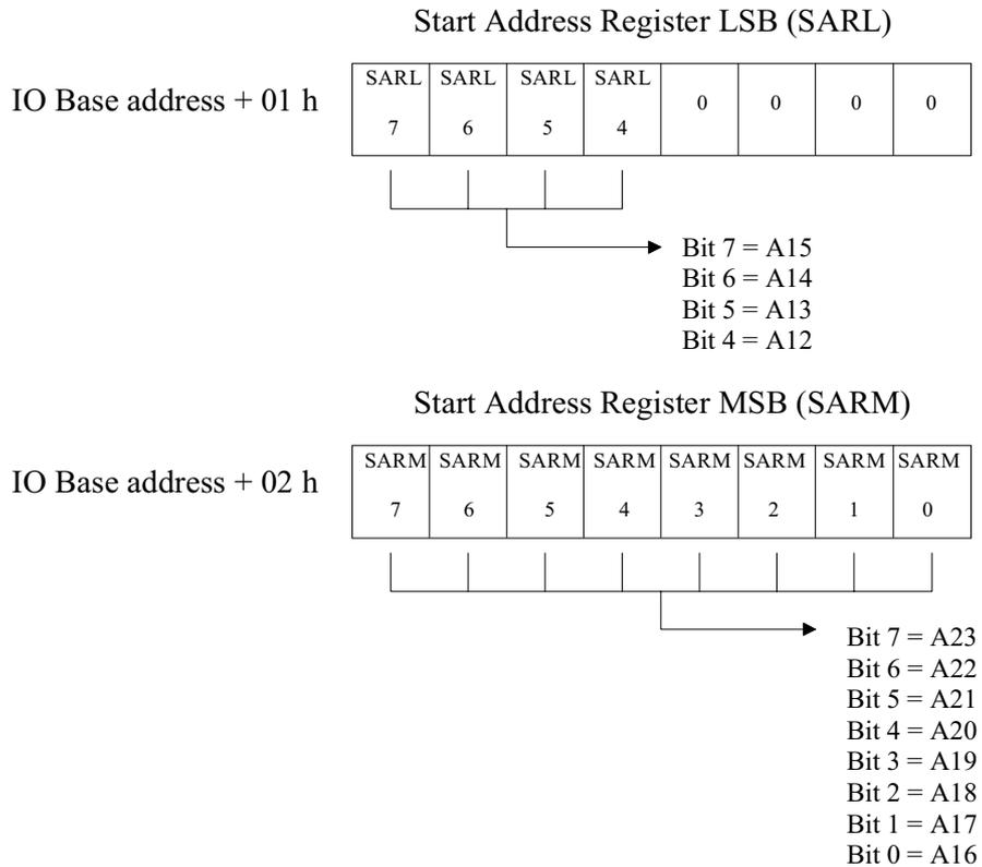
Fig. 9 Start address registers
