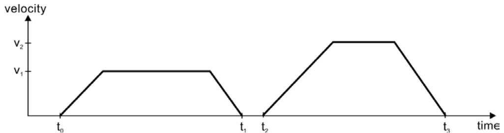
With change\_set\_immediately set to "1" (6), the host instructs the drive to apply a new setpoint immediately after reaching the previous one. The relative timing of the other signals is unchanged. This behavior causes the drive to process the next setpoint X2 in advance, and to hold its velocity when it reaches the target\_position X1 at t1. The drive then moves immediately to the next target\_position X2 that has already been calculated.
