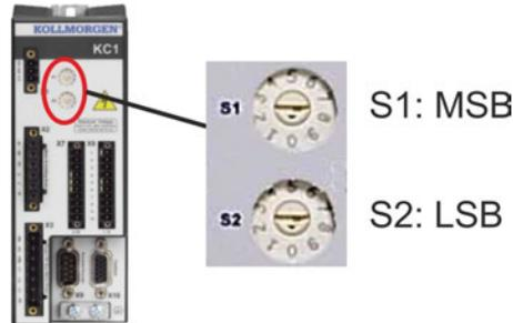
The rotary switches on the front of the KC1 (S1&S2) correspond to the CAN node address. The S1&S2 switches also correspond to the IP address setting of the drive. Both CAN and IP network address schemes have to be configured to account for this dependence if both TCP/IP and CAN networks are running at the same time in an application. Example:
