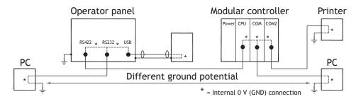
When a PC is connected to the operator panel, the panel's internal 0 V (GND) will be connected to the protective ground via the PC.
