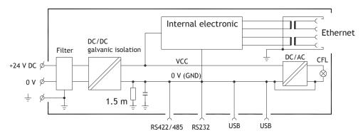
The operator panel has galvanic isolation against the 24 V DC feed but no galvanic isolation between the communication ports for RS232, RS422/485 and USB. Only the Ethernet connection has galvanic isolation.
