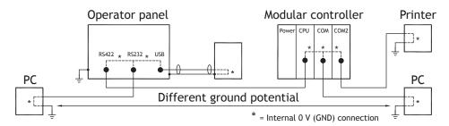
When a PC is connected to the operator panel, the panel's internal 0 V (GND) will be connected to the protective ground via the PC.
