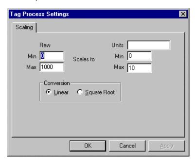
The following properties are part of the Tag Process Scaling properties:
