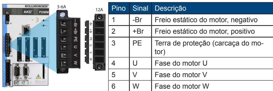
Figura 4. Conector X2, AKD PDMM-xxxx06
