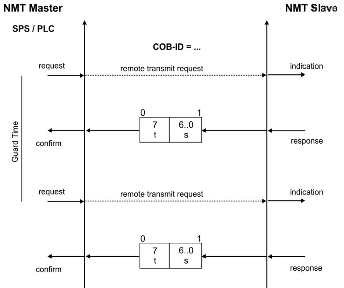
Node guarding is carried out by the Master through RTR telegrams with the COB-ID 700h + slave node address.
