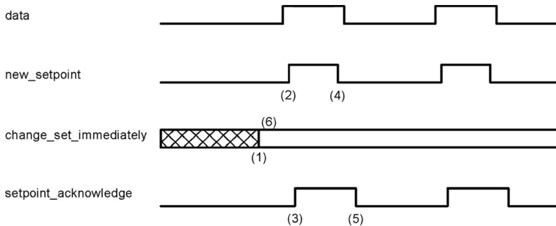
The figures show the difference between the set\_of\_setpoints mode and the single setpoint mode. The initial status of the bit change\_set\_immediately in the control word determines which mode is used. To keep these examples simple, only trapezoidal moves are used.
