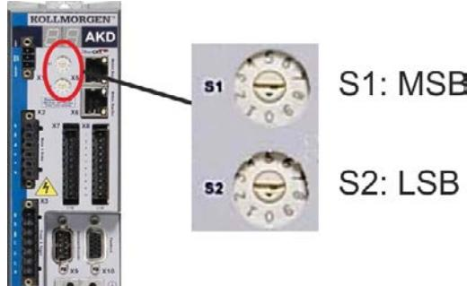
The rotary switches on the front of the AKD (S1&S2) correspond to the CAN node address.
