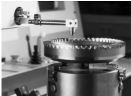
Computerized mapping of gear tooth profile
